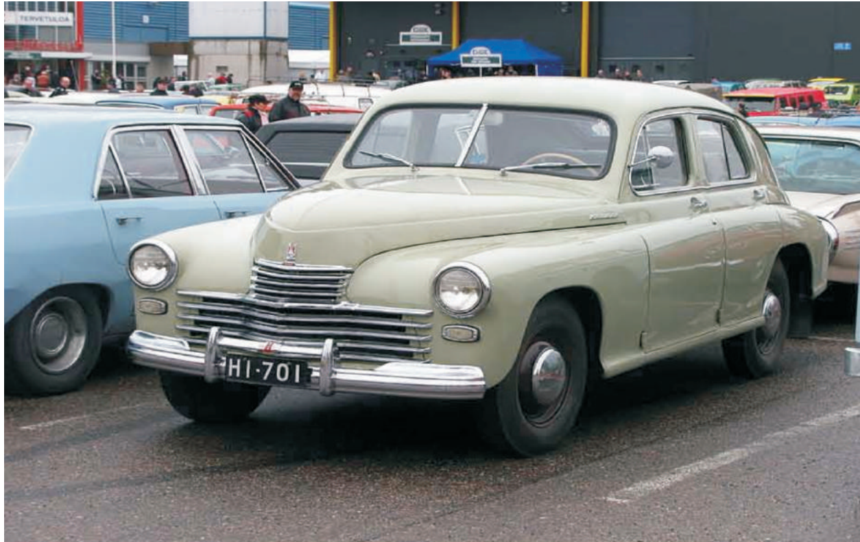
Fig:1946 GAZ-M20 Pobeda one of the first mass produced car with ponton
